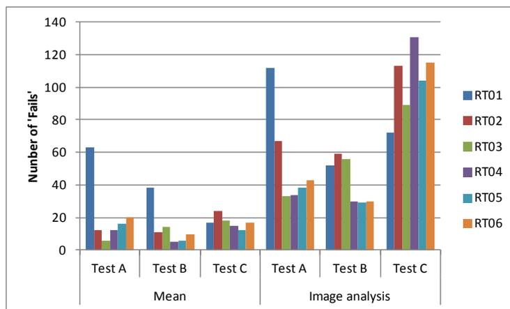
**Figure 5:** Number of 'Fails' recorded for each macroalgae test method from ring tests RT01 through RT06.
