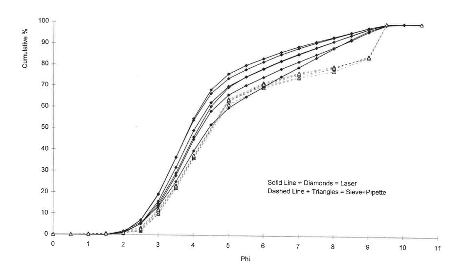
Figure 4. Particle size distribution curves resulting from analysis of sediment sample PS05 by the participating laboratories. Analytical method is indicated by line type; Laser = solid, Sieve = dashed.
