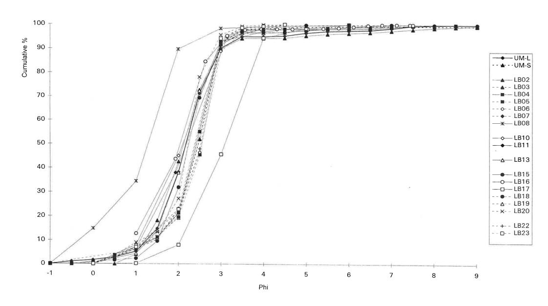
Figure 6. Particle size distribution curves resulting from analysis of sediment sample PS07 by the participating laboratories. Analytical method is indicated.
