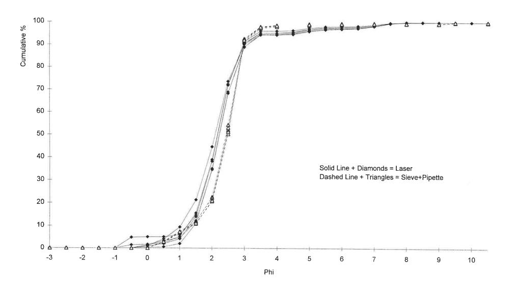
Figure 3. Particle size distribution curves resulting from analysis of twelve replicate samples of sediment distributed as PS07. Six analysed by Laser (solid lines, diamonds) six by Sieve + Pipette (dashed lines, triangles).
