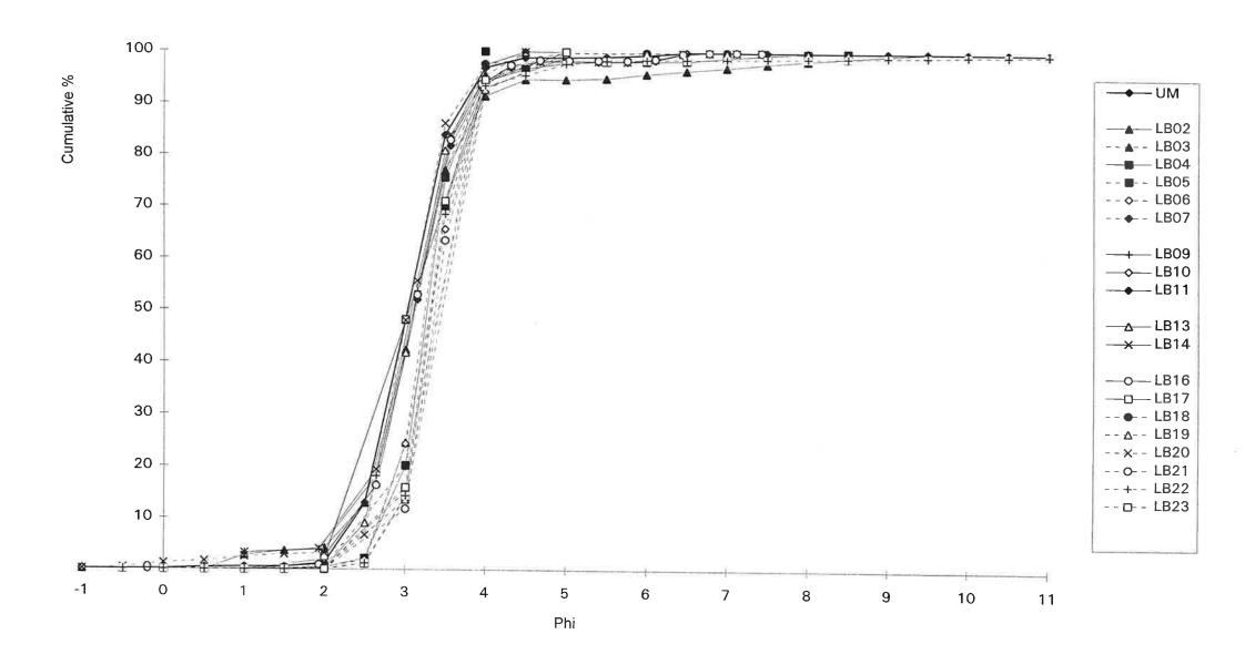
Figure 5. Particle size distribution curves resulting from analysis of sediment sample PS06 by the participating laboratories. Analytical method is indicated by line type; Laser = solid, Sieve = dashed.
