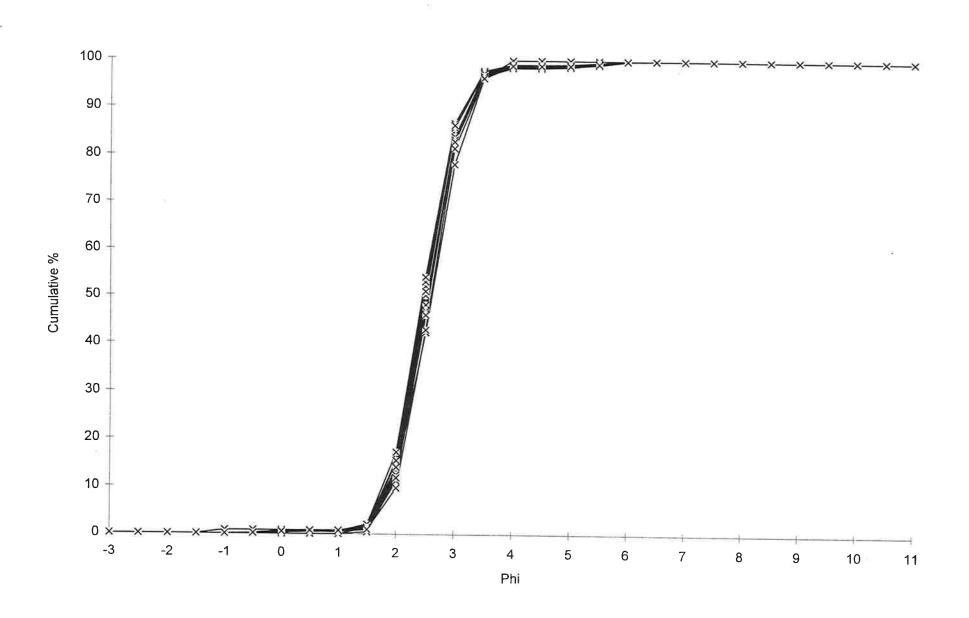
Figure 2. Particle size distribution curves resulting from analysis of twelve replicate samples of sediment distributed as PS06. Six analysed by Laser (solid lines, diamonds) six by Sieve + Pipette (dashed lines, triangles).
