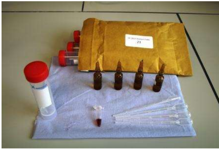
Figure 1: Sample set per participant including sealed vials, lugol's iodine, plastic droppers and 50ml sterilin tubes.
